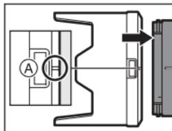
**2 Rotate the lens hood in the direction of the arrow to align mark B (○) on the lens hood with the mark on the tip of the lens.**
